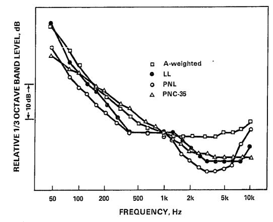
Figure 15. Alternative receiving room spectral shapes used to derive noise isolation curves for the various noise sources shown in Figures 13 and 14 (see text).
