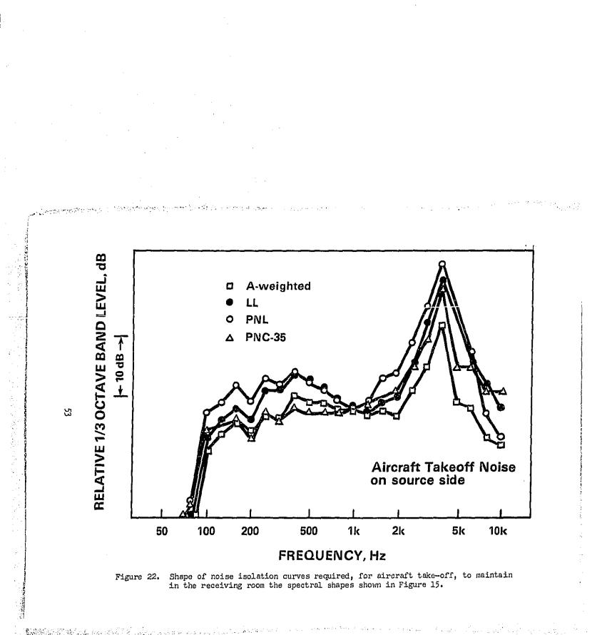
These figures show that when the outdoor noise source has significant high-frequency components (e.g., a large turbofan aircraft on approach), the indoor noise spectrum will be dominated by this frequency region. A rating based upon either loudness level (Mark VII) or noisiness (PNL) would emphasize this high frequency region more than one based upon either a PNC contour or an inverted A-weighting contour.
